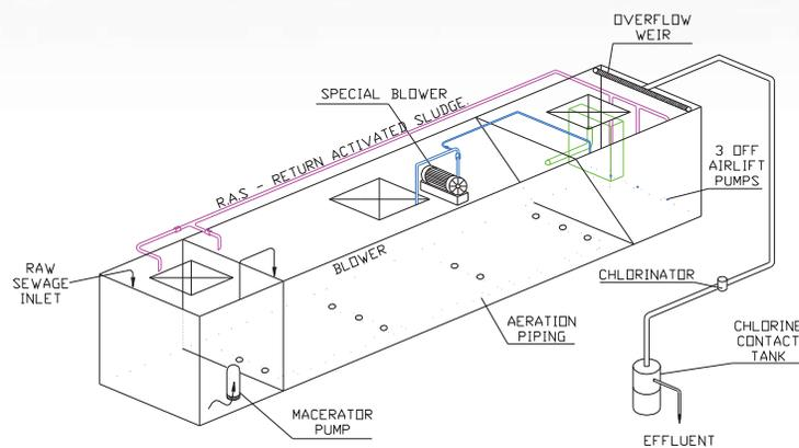
The various plant sections can be identified in the plant above. Some of the other aspects that make the plant different and easier to operate, are:
